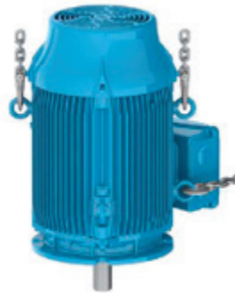
Figure 4.12 - End result: motor placed in vertical position
