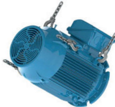
Figure 4.19 - Motor is being rotated to horizontal position
