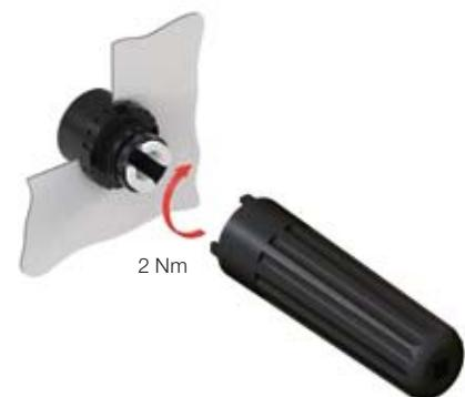
Tighten with the fastening wrench.
